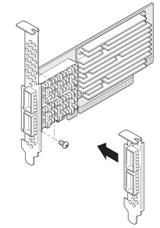
An optional 1PPS bracket and cable assembly, Solarflare part number SOLR-PPS-DP40G, is available for Solarflare QSFP28 server adapters. For detailed fitting instructions, refer to the *Solarflare Server Adapter User Guide*.
