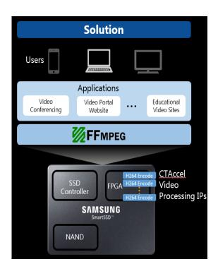
**Fast:** The SmartSSD drive combines a Samsung enterprise-class SSD (Solid State Drive) with a Xilinx FPGA accelerator in one device, enabling fast computation on data directly where it is stored. CTAccel's video processor IP uses this computation power to perform faster H.264 encoding and offload the overloaded data center CPU resources.
