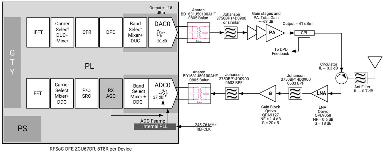
The receiver lineup in this figure shows an example design using standard catalog components that can be used to meet the target requirements listed in the table above. The antenna filter is typically a custom part for mMIMO systems as the size and mechanical fitting is very specific to the design, and, as such, no specific part is indicated.
