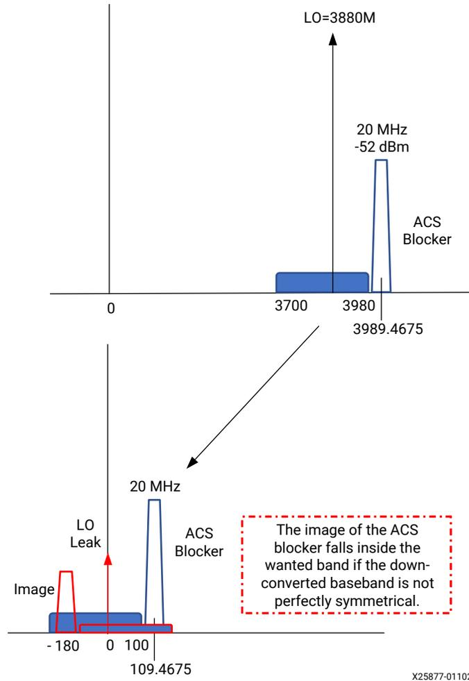
Another operating scenario where the IQ image presents a problem is the ACS requirement for non-contiguous bands. In this situation, the ACS blocker is located in between the non-contiguous bands and its image falls onto one of the operating sub-bands as illustrated in the following figure. Situations like these can severely limit the designer’s frequency planning options.
