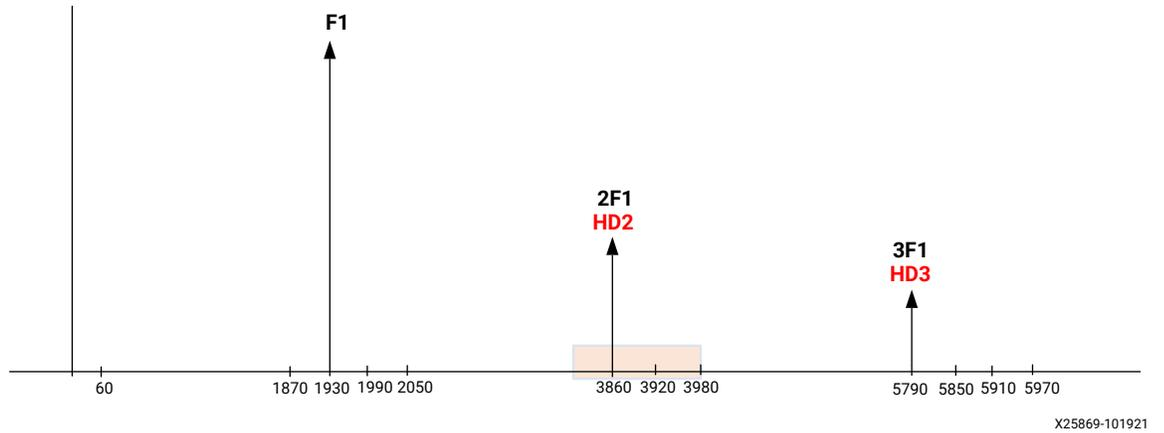
Figure 5: Harmonic Products of Two Wireless Carriers in the PCS Band
