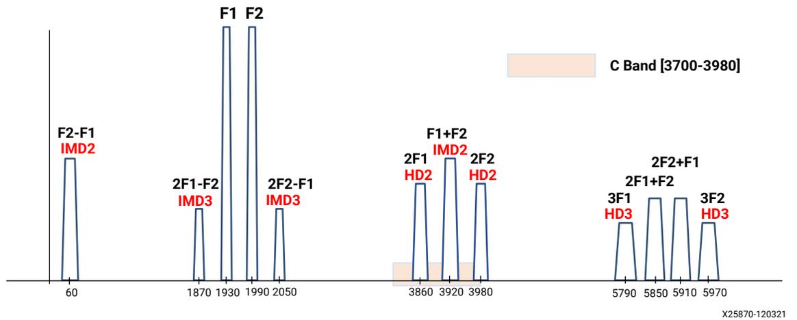
**Figure 6: Actual IMD2/HD2 Measurement on Qorvo QPL9058 ( $V_{DD}=5.0V$ ) LNA at 0 dBm output. OIP2 = 33 dBm at 5V<sub>DD</sub>; OIP2 = 29 dBm at 3.3V<sub>DD</sub>.**
