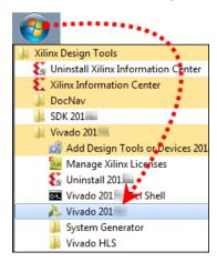
Figure 1-1: Launching the Vivado Design Suite from the Start Menu
