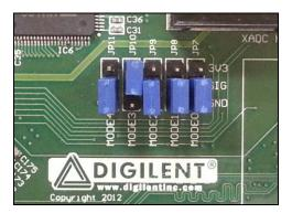
Figure 10-22: Jumper Setting for QSPI Boot (ZedBoard)
