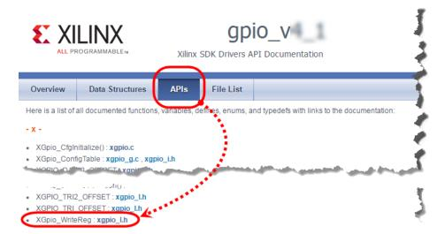
Figure 5-17: Locating the XGpio\_WriteReg API
