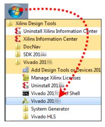
Figure 12-1: Launching the Vivado Design Suite from the Start Menu
