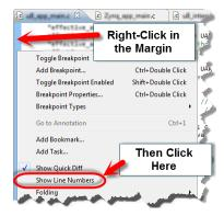
Figure 4-15: Enabling Line Numbering
