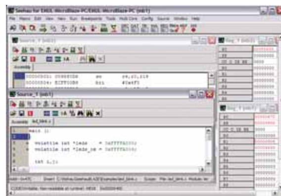
Figure 7 – Multi-core display with two MicroBlaze processors
