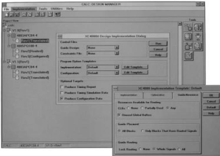
critically-timed logic and graphically plan the data flow. Placement is performed at a high level using the designs' hierarchy and a floorplan of the target device. Floorplanning also allows optimal use of specialized FPGA architectural structures like high-speed distributed RAM and internal three-state buffers. Users needing to maximize performance can easily implement a detailed floorplan employing proven optimization techniques like bus interleaving, register grouping and I/O pin alignment.
