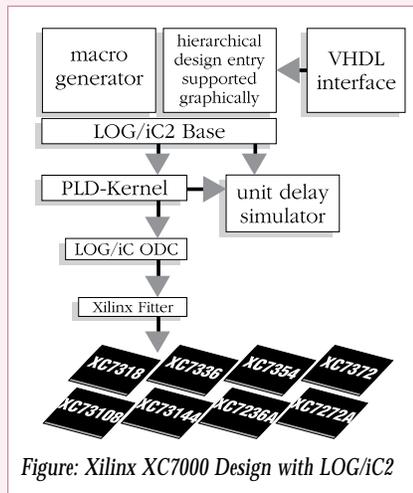
Figure: Xilinx XC7000 Design with LOG/iC2
