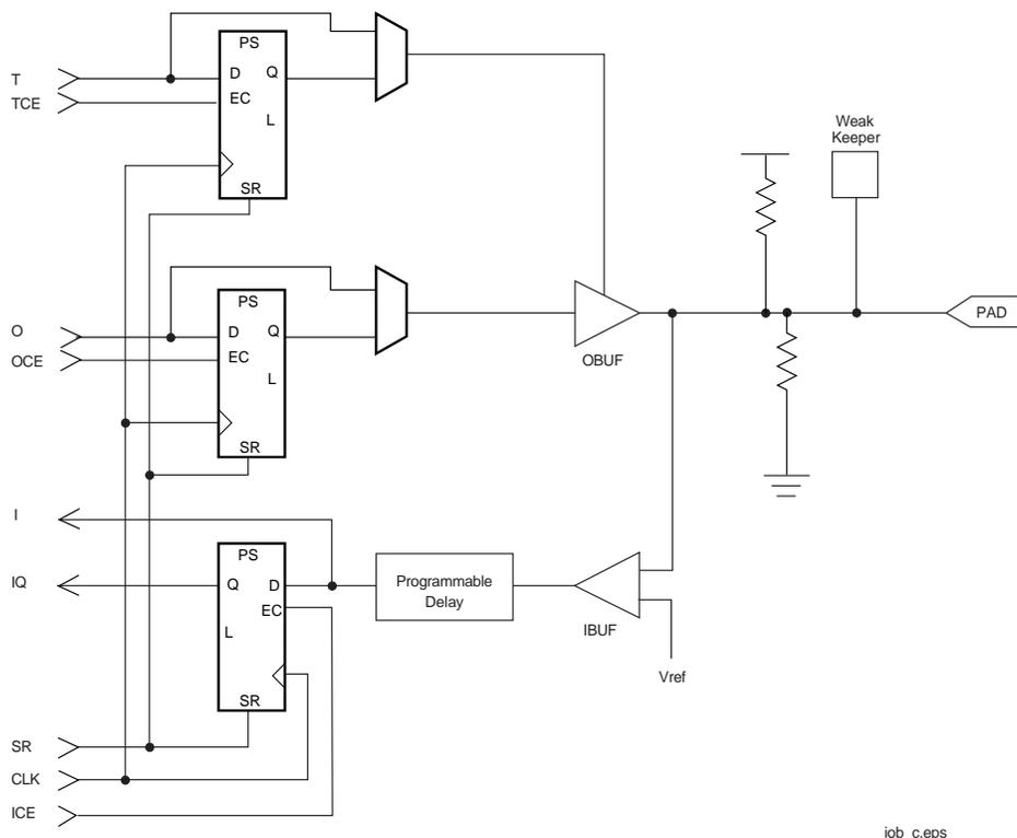
Figure 2: Virtex Input/Output Block (IOB)
