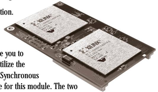
Example VHDL functions that enable you to quickly and easily utilize the onboard FIFOs and Synchronous DRAMs are available for this module. The two independent SDRAMs allow you to implement a versatile arrangement of data analysis and manipulation techniques.
