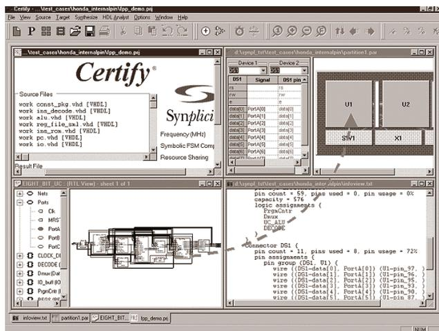
*Partition by dragging and dropping HDL modules to different FPGAs*
