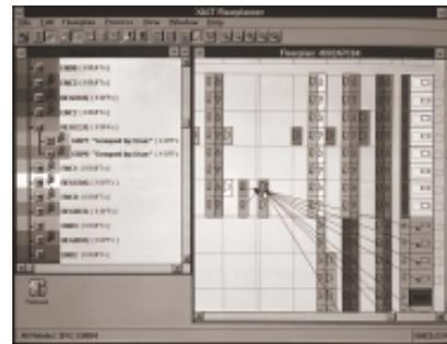
layout process, thus simplifying the increasingly complex problem of logic placement. Advanced programmable logic designers found that by "seeding" the placement of a small portion of a design, they could improve circuit performance by up to 25%, and cut place and route run times in half. Furthermore, the Floorplanner proved to be an excellent tool for analyzing a design's logic and routing density, providing insight into the suitability of a design for future enhancements.
