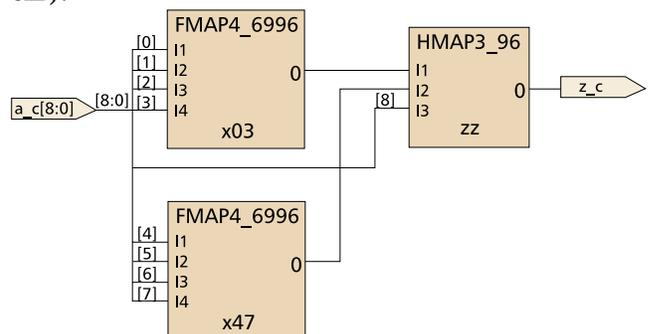
**Virtex family: Replace the xc\_rloc value to include the slice also:**
