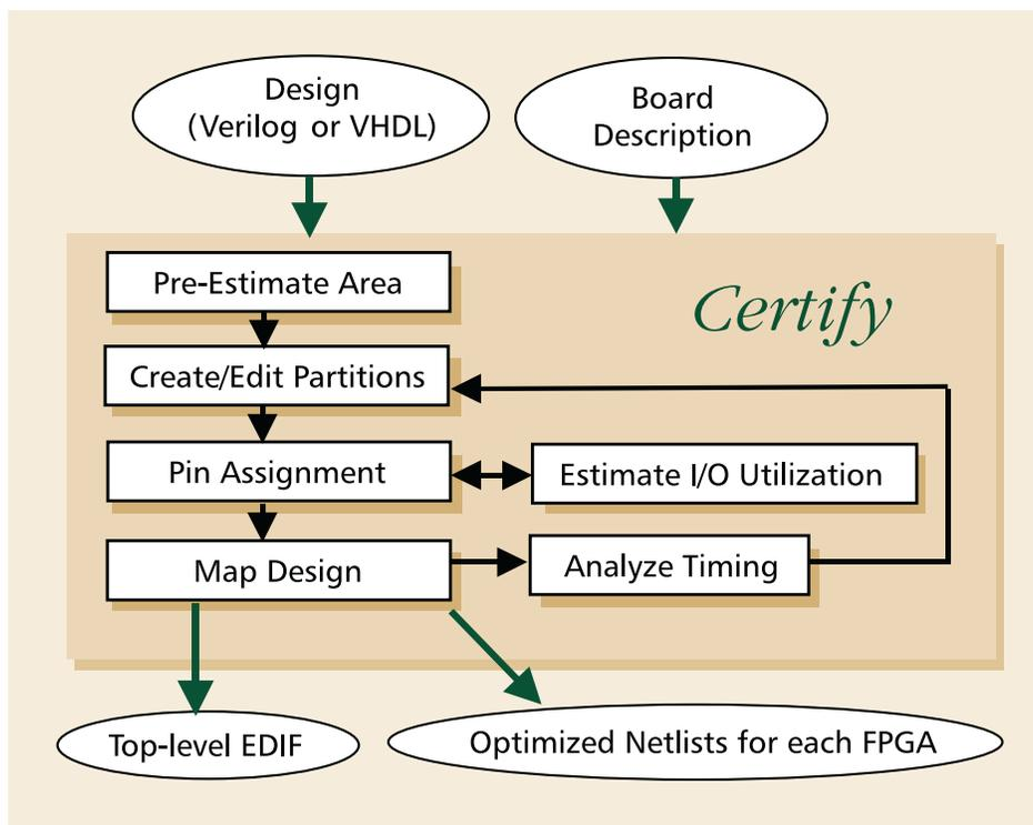
*Of course, the most effective changes are major changes to the circuit topology that derive from a deep understanding of the design. This is the technique used by Certify's unique partition-driven synthesis algorithms to produce optimal results.*
