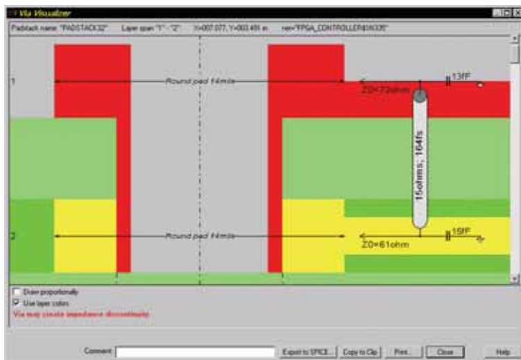
Figure 3 – The HyperLynx Via Viewer shows a low-loss blind via. Also shown is the via capacitance, characteristic impedance, and signal propagation delay through the via. Via “what-if” exploration is now possible during pre-layout analysis, enabling you to perform loss and eye-quality trade-offs with different via combinations.
