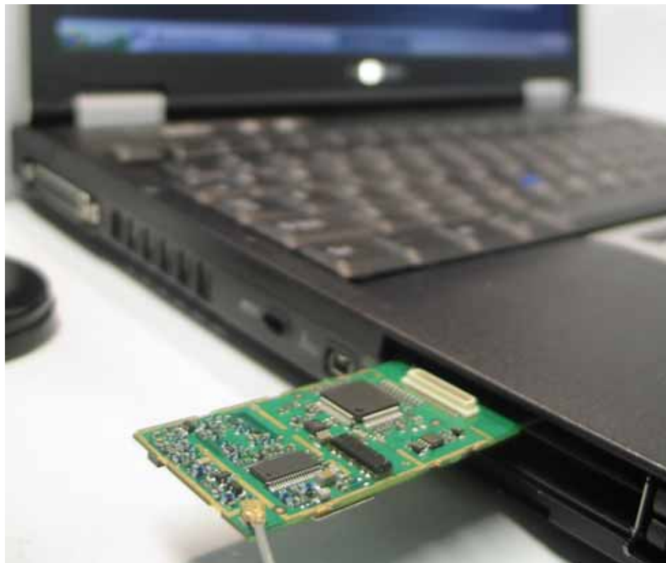
Figure 2 – The Philips/Xilinx CES 2006 DVB-T ExpressCard/34 module demonstrates live digital TV reception on a notebook computer.
