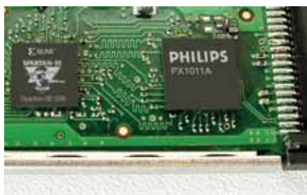
Figure 3 – Xilinx Spartan-3E FPGA and Philips PX1011A on a DVB-T ExpressCard/34 demonstrator
