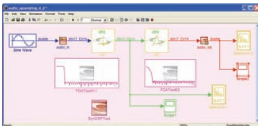
Figure 2 – Modules from the Synplify DSP block set and Simulink FDA tool implement the sampling rate converter. Simulink block set elements perform verification.
