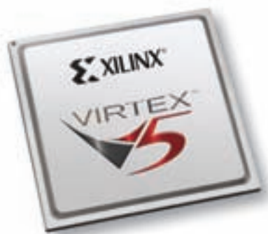
Figure 2 – High-performance FPGA families, such as the Xilinx Virtex-5 family, have common elements for logic, DSP, memory, and I/O, with a common package strategy enabling technology insertion at the component level.
