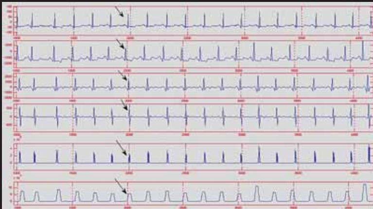
Figure 1 — Input ECG and filtering stages output, from top to bottom: original signal, low-pass output, high-pass output, derivative output, squaring stage output, moving window integrator output. The arrow indicates the position of the QRS complex.
