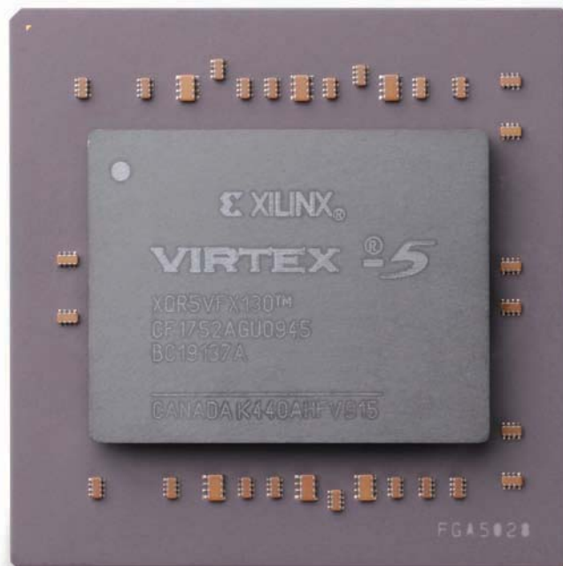
Figure 1 – Xilinx built its latest space-grade FPGA, the Virtex-5QV, to be rad-hard.
