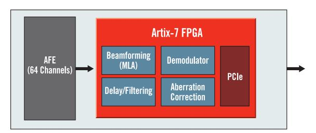
Designers can deploy a fully programmable 64-channel portable ultrasound implementation that scales up to 196 or 256 channels for high-end cart solutions or down to 32 channels for hand-held form factors.
