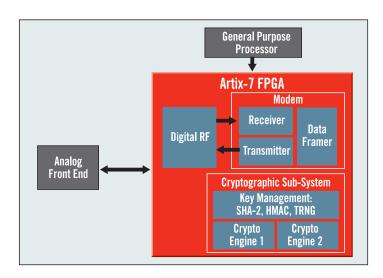
The Artix-7 FPGA delivers the industry's most integrated Type-1 single-chip cryptography (SCC) solution for superior, secure SWaP-C results. Extensive DSP resources allow for waveform processing capacity to integrate both the modem and cryptographic engine on a single chip.
