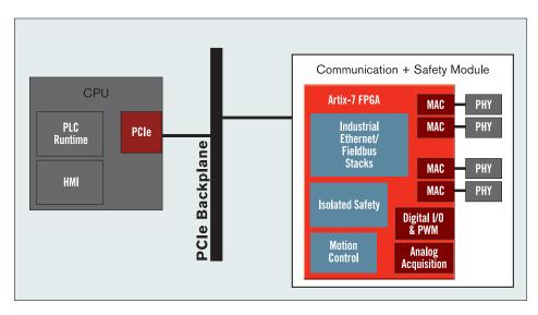
Employing the Artix-7 FPGA and Xilinx IP solutions enables a smaller form factor programmable logic controller (PLC) with greater flexibility, lower BOM cost, and total power consumption compared to traditional architectures. Serving as a companion device to the main processor, the FPGA replaces communication expansion modules.
