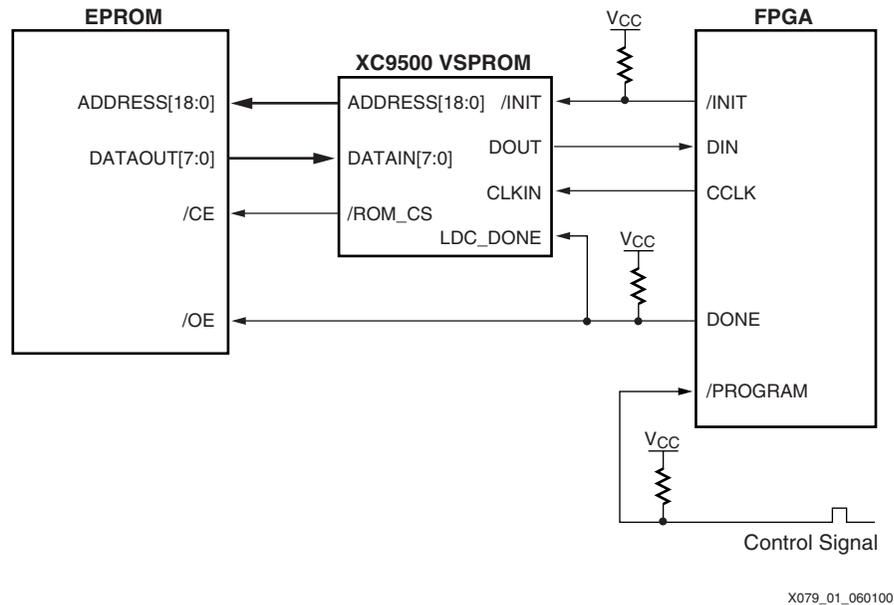
Figure 1: XC9500 VSPROM Design Interface to FPGA
