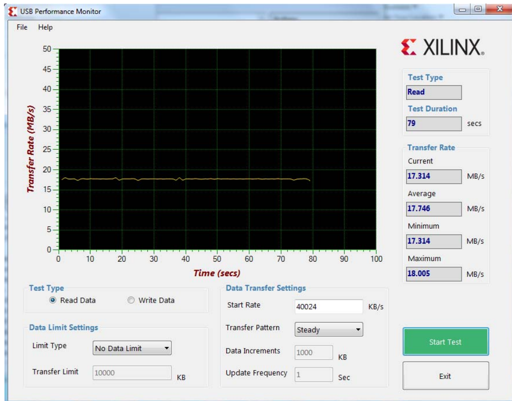
Figure 6: Performance Measurement for Bulk Transaction (40024 KB/s start rate)
