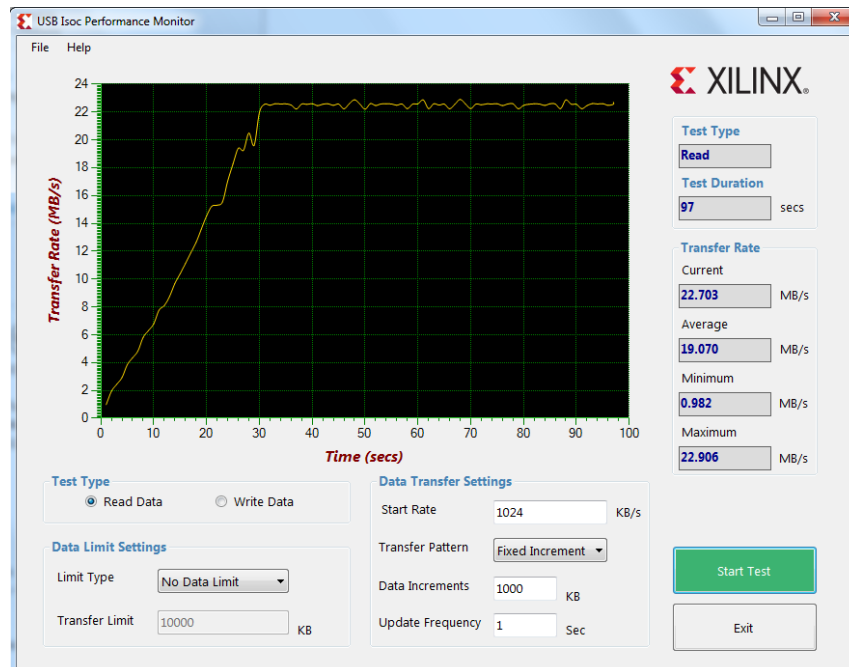
Figure 9: Performance Measurement for Isochronous In Transaction
