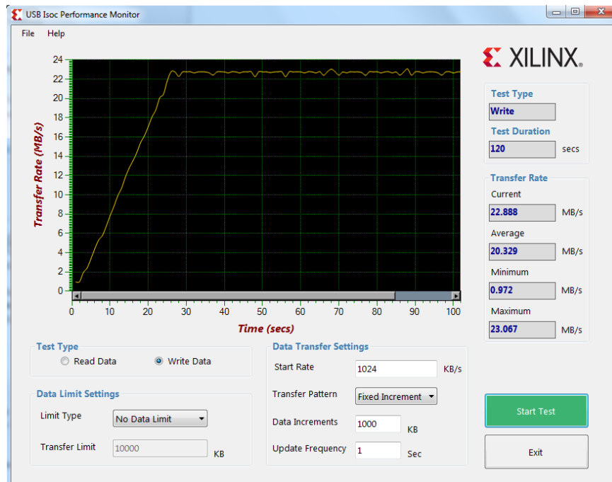
Figure 8: Performance Measurement for Isochronous Out Transaction
