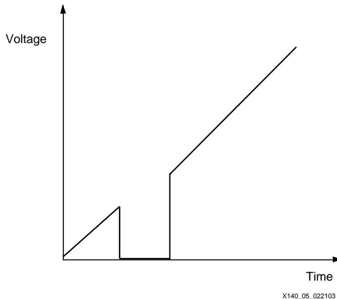
Figure 5: Macrocell Voltage versus Time During Power Up
