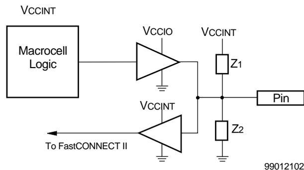
Figure 1: Simplified XC9500XL I/O Structure
