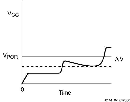
Figure 7: Non-monotonic  $V_{CC}$
