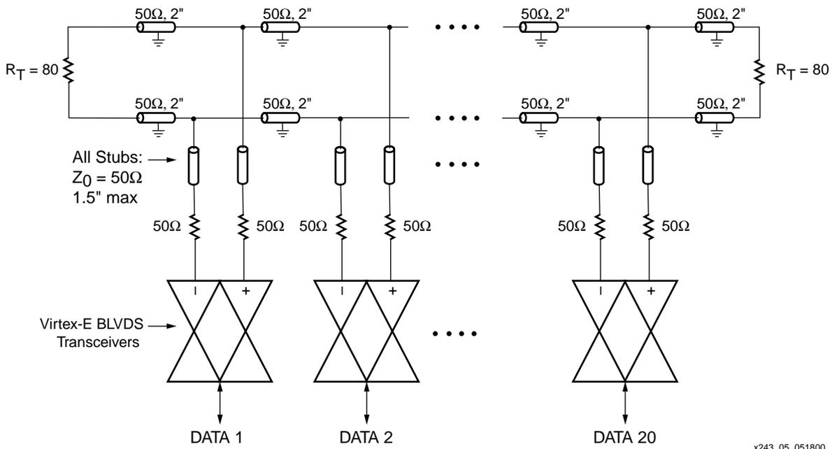
Figure 5: 20-Load Multipoint LVDS Using Virtex-E Devices
