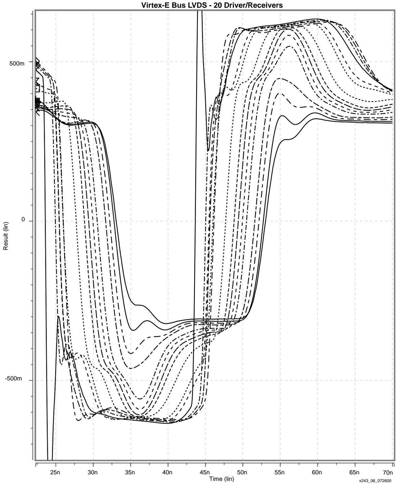
Figure 6: Simulation Waveforms for 20-Load Virtex-E Multipoint LVDS
