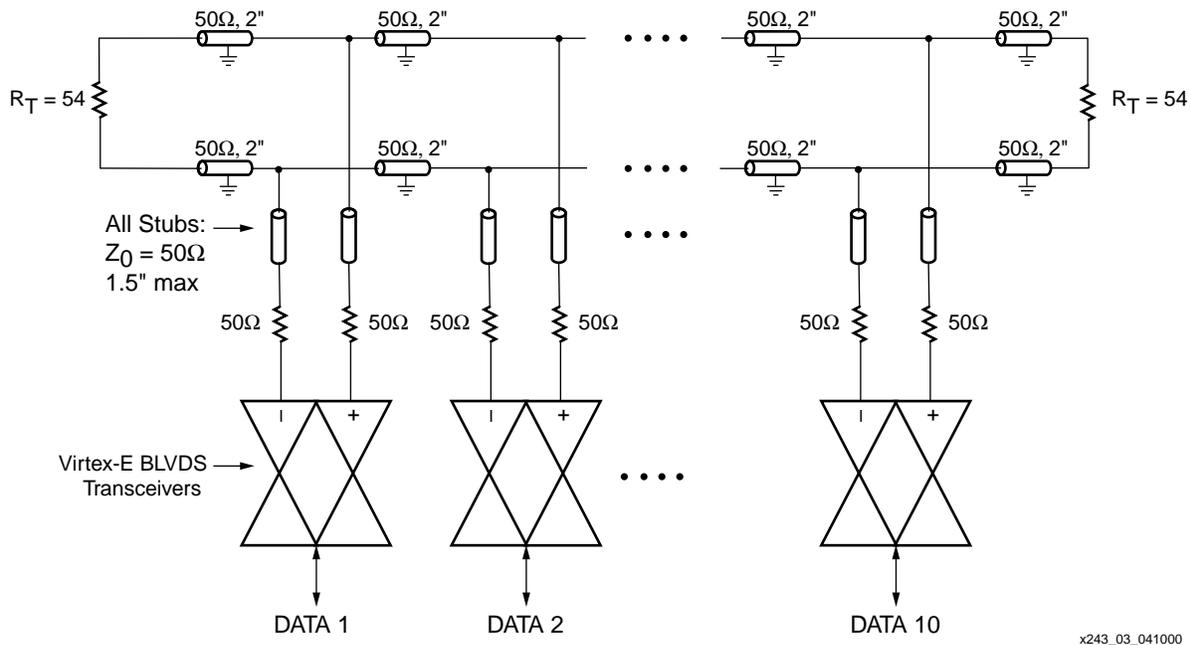
Figure 3: 10-Load Multipoint LVDS Using Virtex-E Devices
