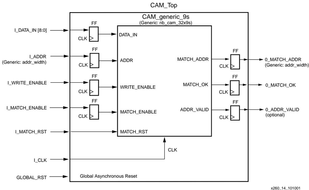
Figure 14: CAM Design Top Level Block Diagram
