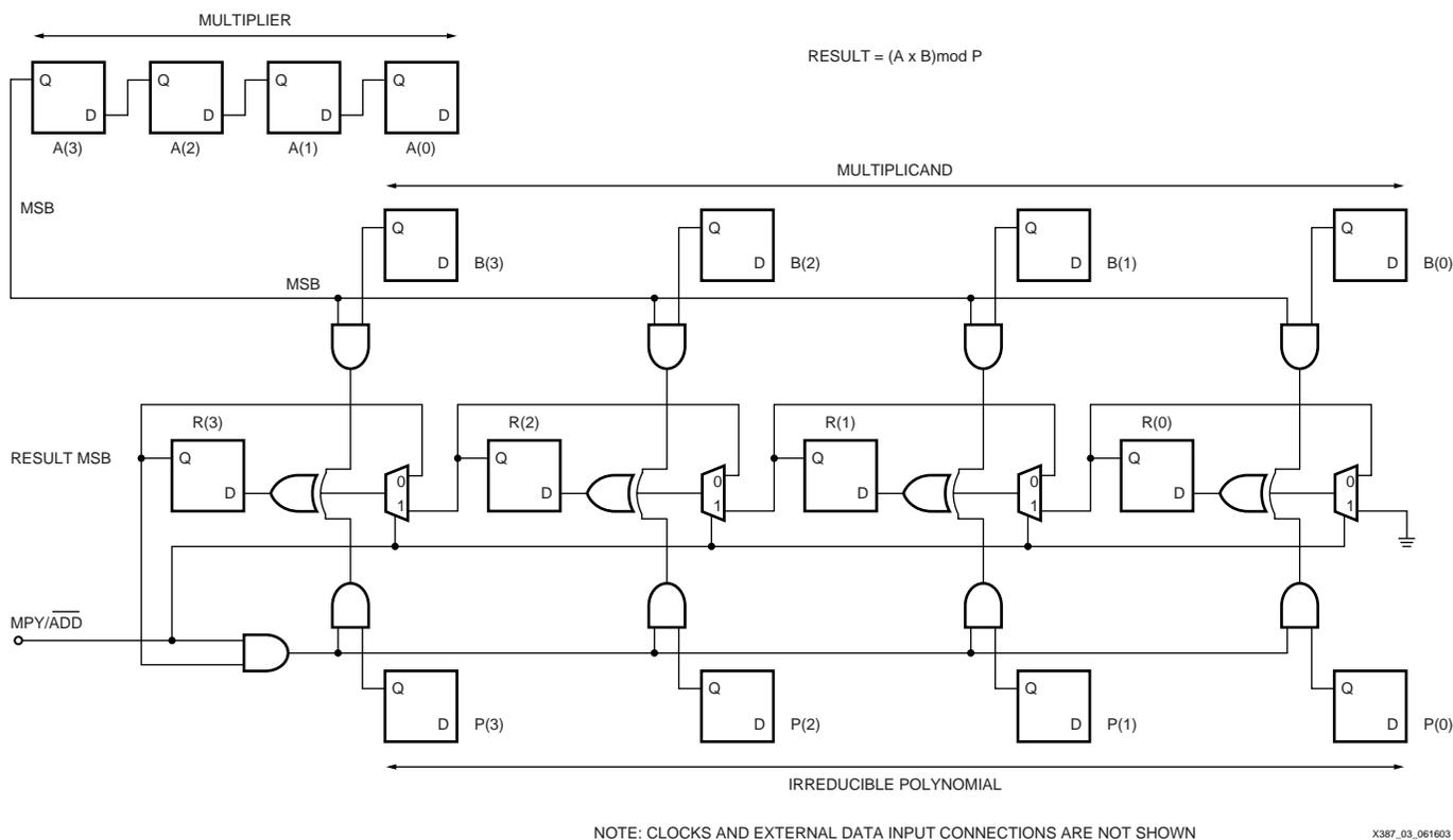
Figure 3: 4-Bit GF (2<sup>2</sup>) Multiplier
