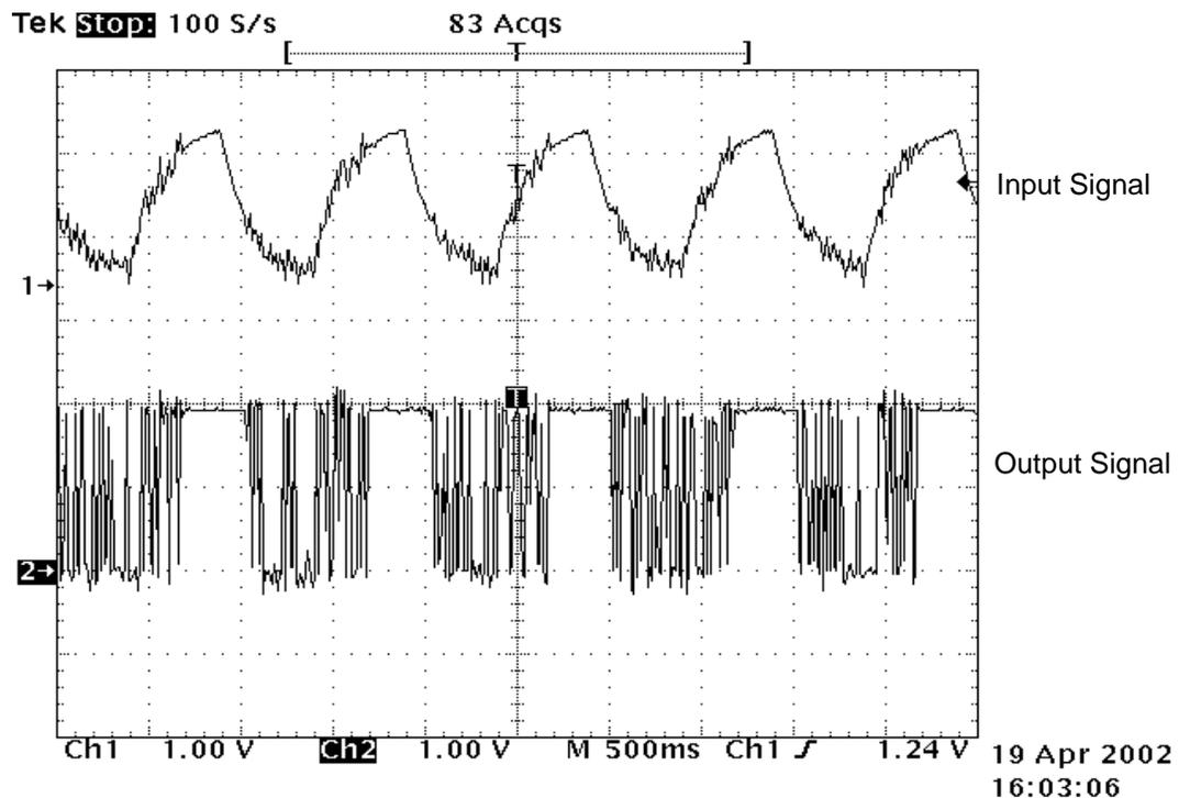
*Figure 5: Non-Schmitt Waveforms*
