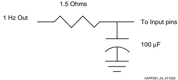
*Figure 4: Low Pass Filter for Schmitt Trigger Demo*
