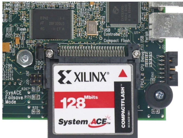
Figure 1: ML40x Evaluation Platform with CF Card
