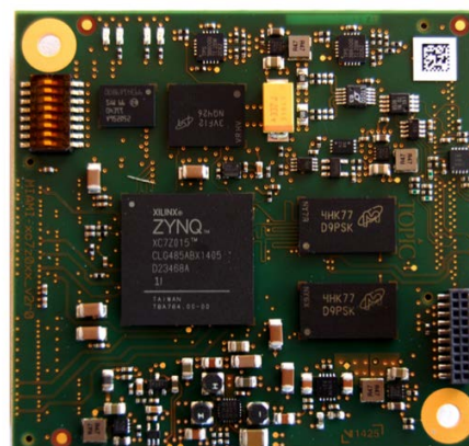
Topic Embedded compact, Zynq-based Miami SOM measures only 65x68.4mm
