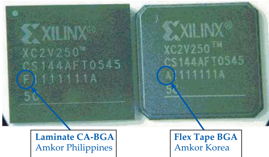
Figure 1: Package Top Mark Showing Assembly Site Code
