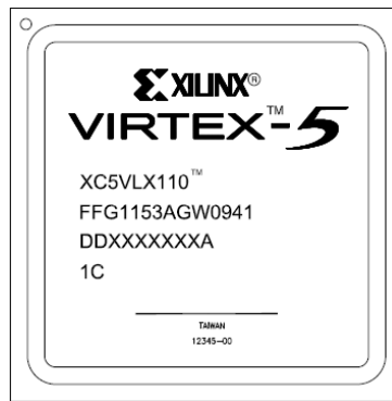
Figure 2: New Marking (Laser)
