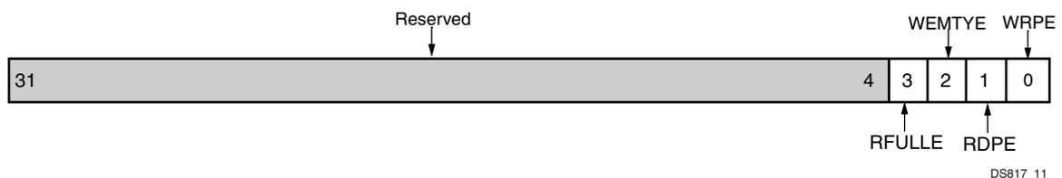
Figure 2-3: IP Interrupt Enable Register (IPIER)
