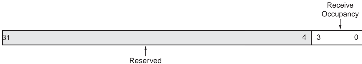
Figure 13: Receive FIFO Occupancy Register (RX_FIFO_OCY)
