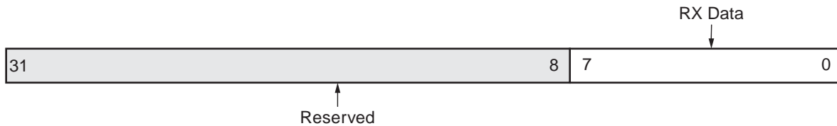
Figure 9: Receive FIFO (RX_FIFO)
