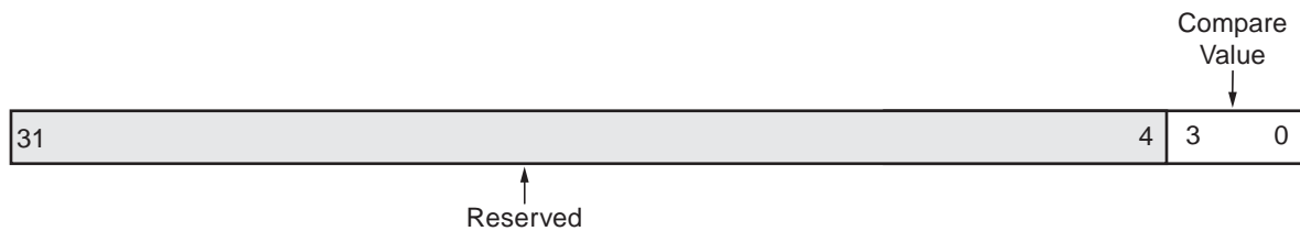
Figure 14: Receive FIFO Programmable Depth Interrupt Register (RX_FIFO_PIRQ)
