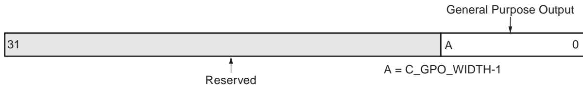
Figure 15: General Purpose Output Register (GPO)
