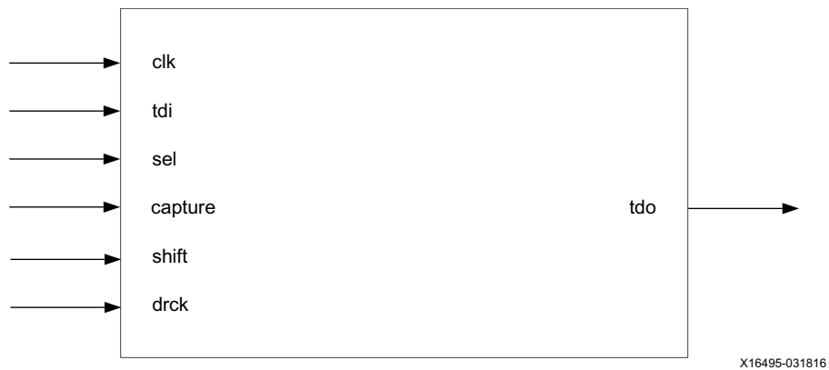
Figure 1-1: Debug Bridge Configured with From_BSCAN_to_DebugHub Mode
