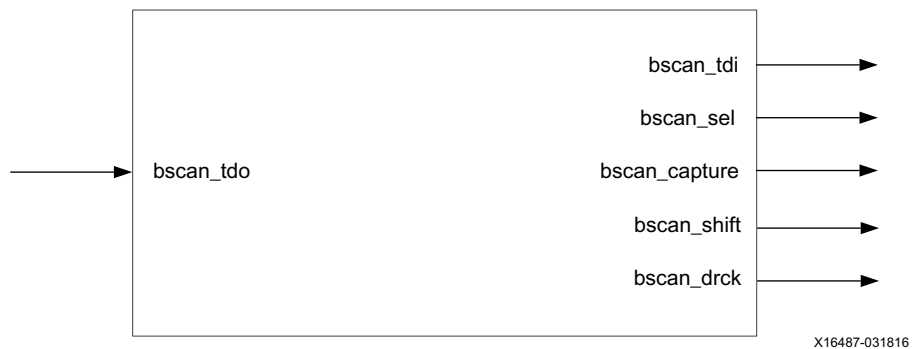
Figure 1-2: Debug Bridge Configured with BSCAN_primitive Mode
