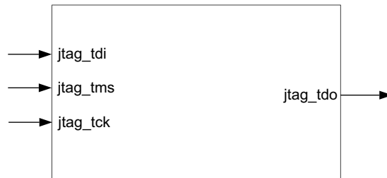
Figure 1-7: From_JTAG_to_BSCAN Mode Port Diagram
