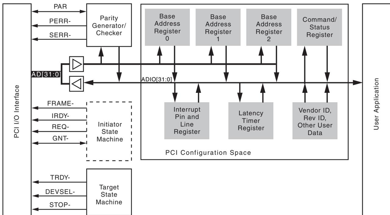
Figure 1: Initiator/Target Core for PCI Block Diagram
