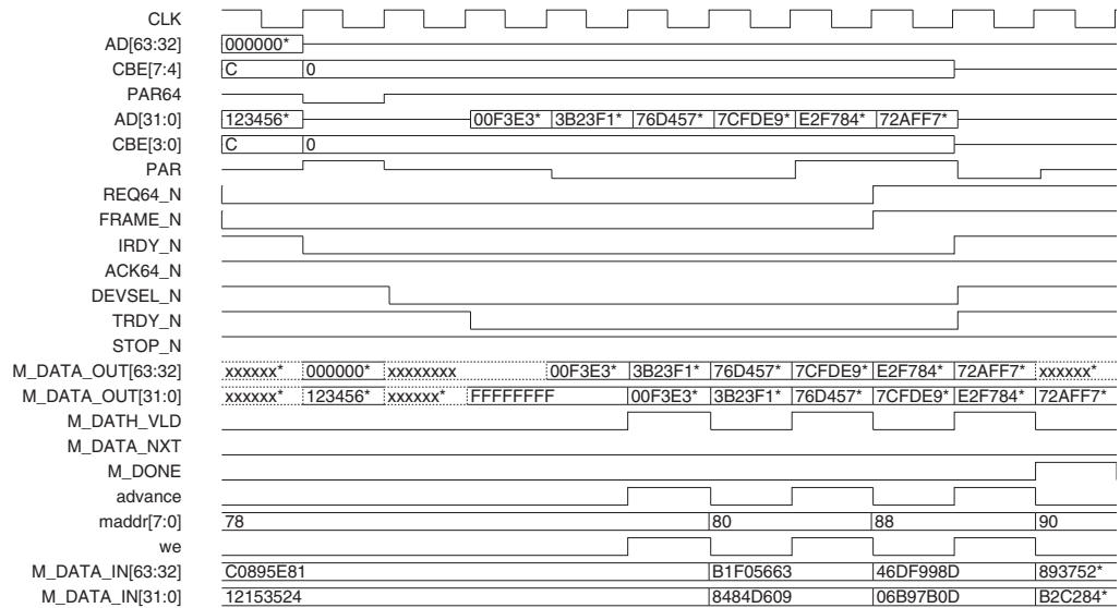
Figure 10-6: PCI Burst Read, 64-Bit Request, 32-Bit Target
