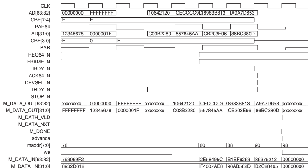
Figure 10-3: PCI-X Burst Read, 64-Bit Request, 64-Bit Target
