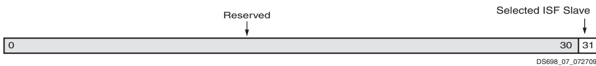
Figure 7: SPI Slave Select Register (C_BASEADDR + 0x70)
