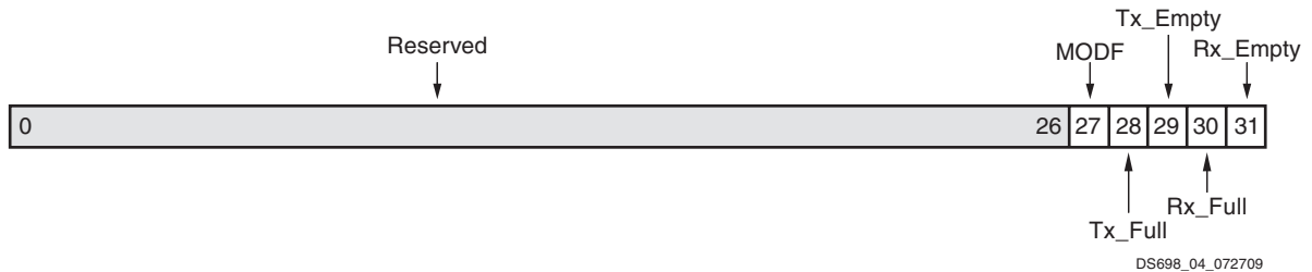
Figure 4: SPI Status Register (C_BASEADDR + 0x64)
