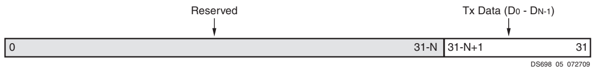
Figure 5: SPI Data Transmit Register (C_BASEADDR + 0x68)
