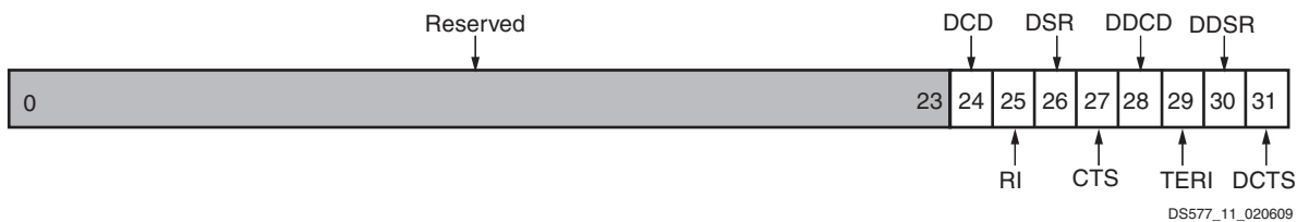
Figure 11: Modem Status Register (MSR)
