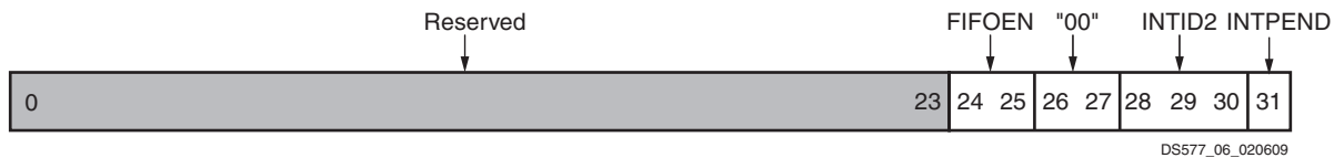
Figure 6: Interrupt Identification Register (IIR)
