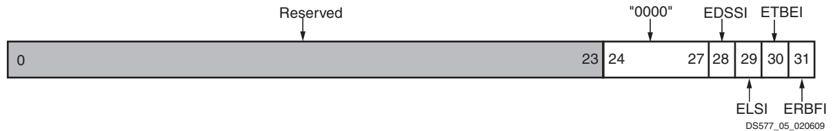
Figure 5: Interrupt Enable Register (IER)
