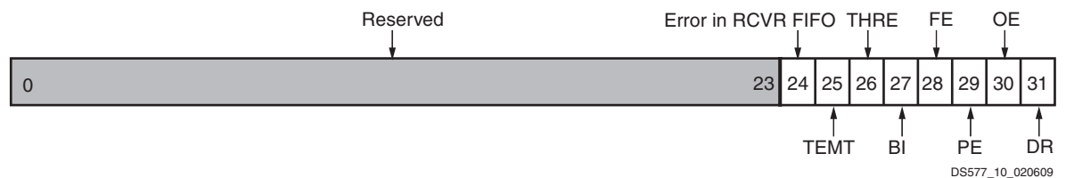
Figure 10: Line Status Register (LSR)
