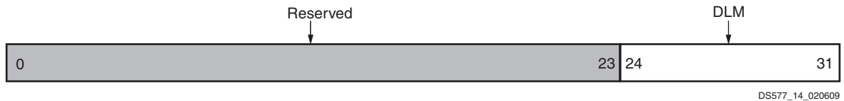
Figure 14: Divisor Latch (Most Significant Byte) Register
