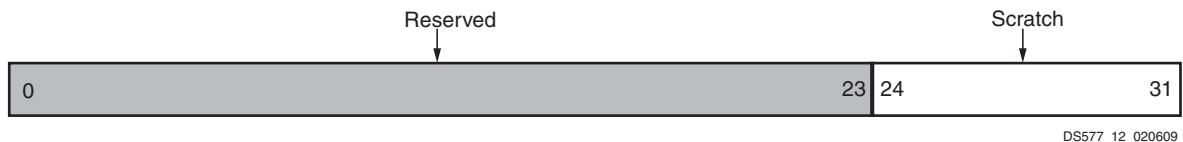
Figure 12: Scratch Register (SCR)
