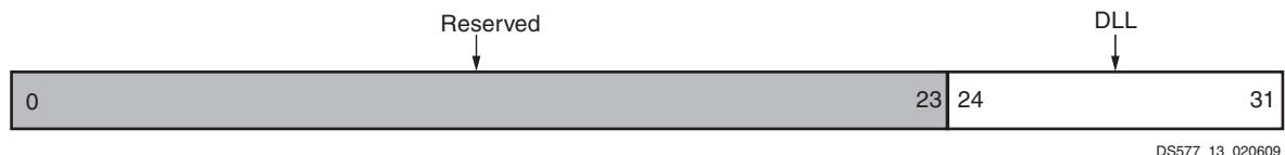
Figure 13: Divisor Latch (Least Significant Byte) Register
