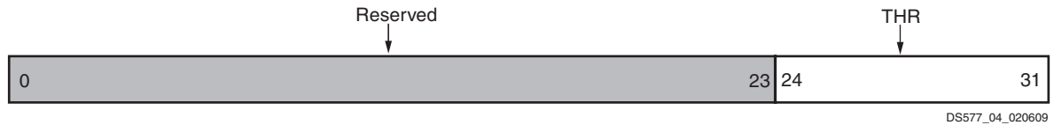
Figure 4: Transmit Holding Register (THR)
