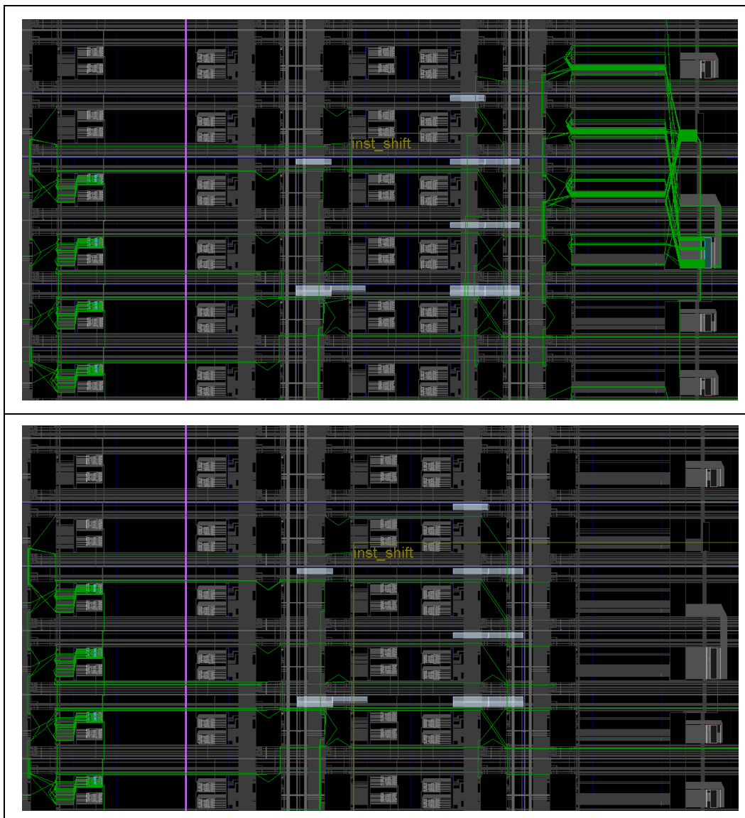
Figure 8: The inst_shift module before (top) and after (bottom) update_design -black_box
