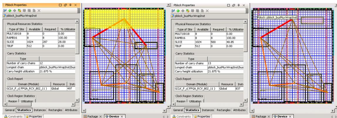
**Figure 12: Resource Utilization Feedback to Aid Floorplanning**
