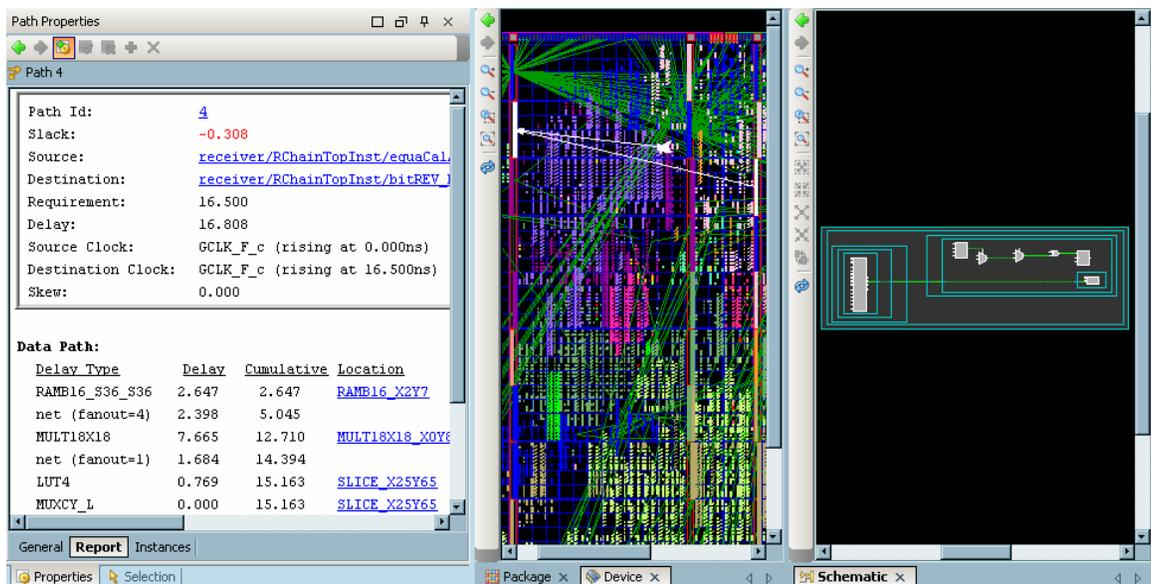
**Figure 7: Visual Feedback of Timing Critical Paths**
