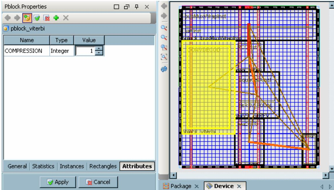
**Figure 11: Applying Compression**
