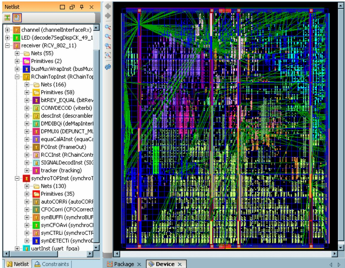
**Figure 5: Placement Analysis through Selective Logic Highlighting**
