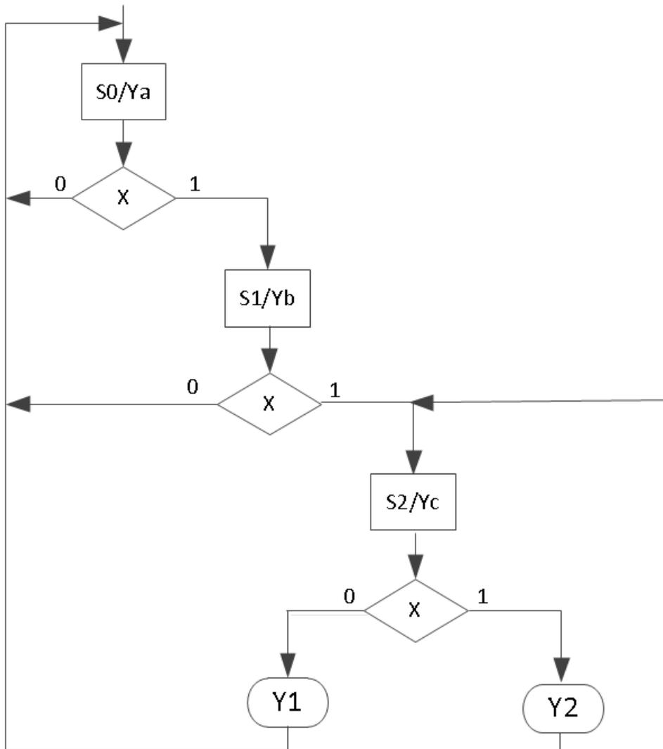
Once the ASM chart is determined, the conversion to HDL is straight forward. A `case` statement can be used to specify what happens in each state. Each condition box corresponds directly to an `if` statement (or an `else if`). The following code represents the functionality of the above ASM chart.
