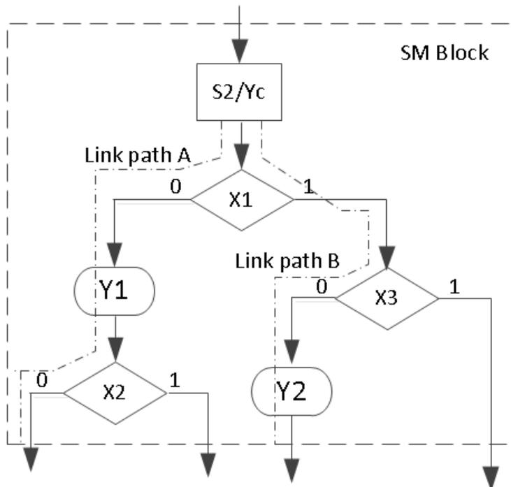
Let us consider an example of a state graph of a sequential network shown below. This state graph has both Mealy and Moore outputs. The output Y1 and Y2 are the Mealy outputs and so should be conditional outputs. The Ya, Yb, and Yc are the Moore outputs so they should be part of state box. Input X can either be "0" or "1" and hence it should be part of the decision box.
