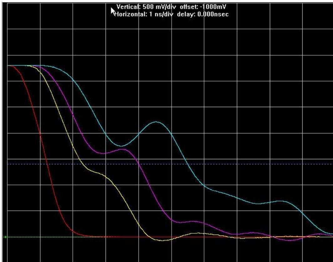
Figure 5: Daisy Chain Configuration, LVCMOS33 6 ma Fast Slew
