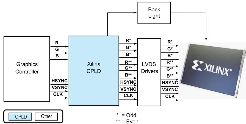
Figure 5: Timing Controller
