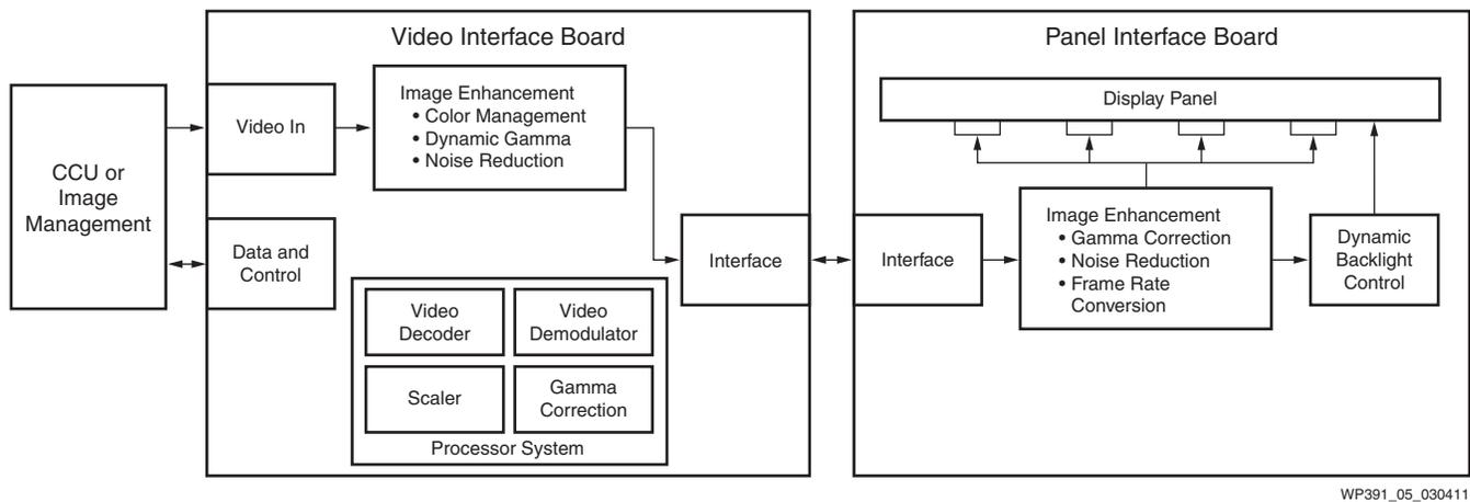
Figure 5: Medical Display Block Diagram
