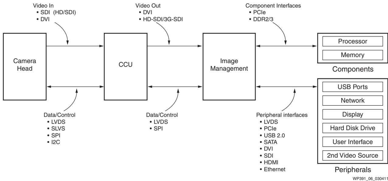
Figure 6: Common Interfaces in Endoscope Systems
