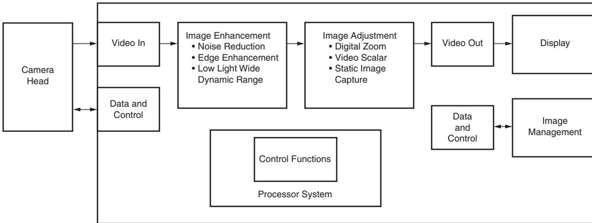
Figure 3: CCU Functional Diagram
