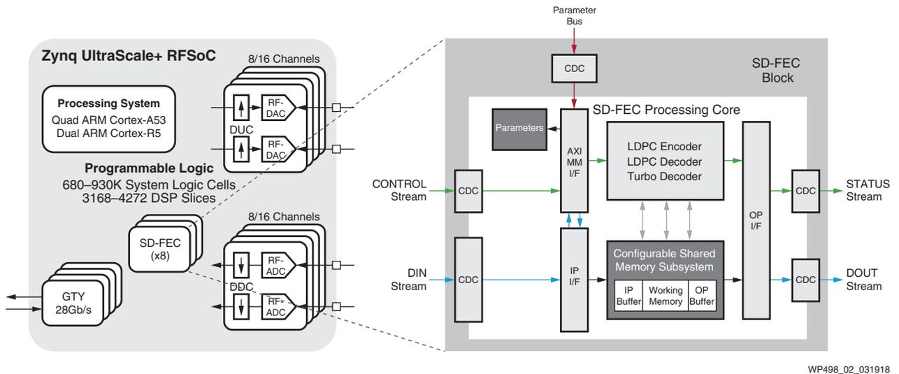
Figure 2: SD-FEC Block Diagram
