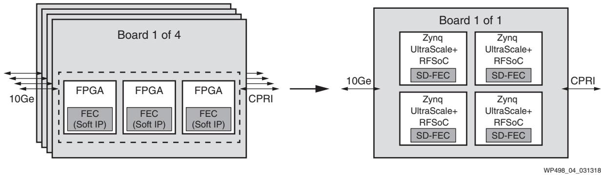
Figure 4: SD-FEC Enables Reduction in PCB Count
