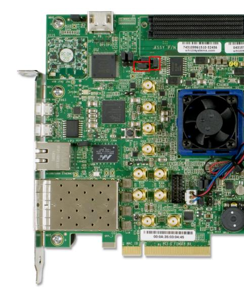
➤ Attach the FMC XM107 board to the FMC HPC connector (J22)
