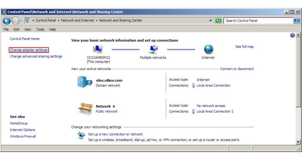
➤ Right-click on the Gigabit Ethernet Adapter that you will be using for this test and select Properties
