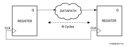
The default Setup and Hold relationships that are resolved by the Static Timing Analysis (STA) tool are shown in the following figure.
