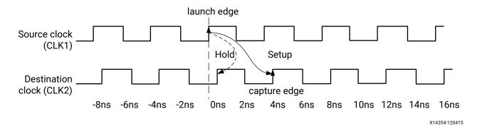
In the case of negative phase-shift, as shown in the following figure, between the two clock domains, the launch and capture edges used for the setup and hold checks are similar to those from the previous section (single clock domain, no phase-shift).
