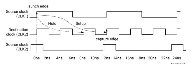
Figure 75: Setup=3, Hold Moved Accordingly
