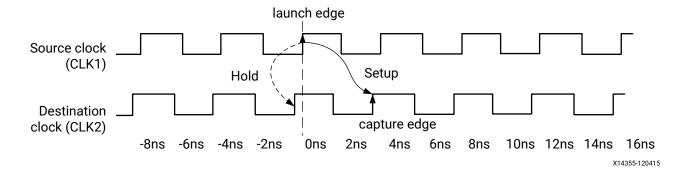
For a negative phase-shift, a Multicycle constraint is typically not needed to counter-balance the effect of the phase-shift. An exception occurs if the phase-shift is so large that the clock launch or capture edges must be adjusted to keep realistic setup and hold requirements.
