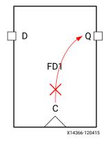
The process of stopping the propagation of the timing to create a valid startpoint is called path segmentation. Path segmentation affects both max and min delay analysis. Path segmentation also affects any timing constraint going through those nodes (FD1/C and FD1/Q).
