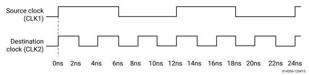
The setup and hold relationships that are resolved by the STA tool when no multicycle is applied are shown in the following figure.
