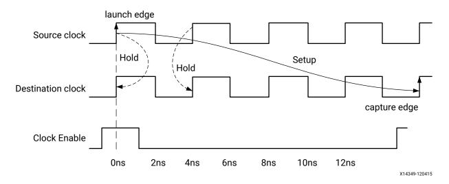
Figure 64: Multicycle Path with Setup Multiplier of Four (4)
