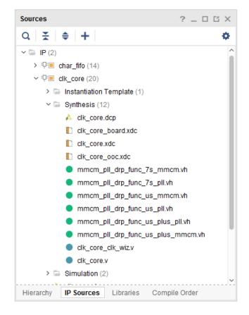
Figure 3: XDC Files in the IP Sources
