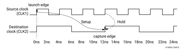
**IMPORTANT!** For a FAST-to-SLOW clock domain crossing, define a setup multiplier of N against the launch clock (-start) with a hold multiplier of N-1 (most common case). See the following example:
