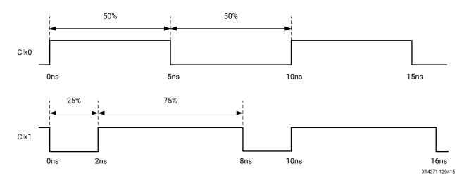
Figure 49: Clock Waveforms Example
