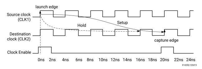
Figure 65: Setup=5, Hold Moved Accordingly
