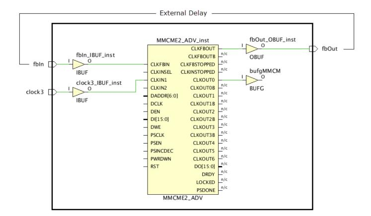
Figure 17: Typical MMCM External Feedback Path Circuit
