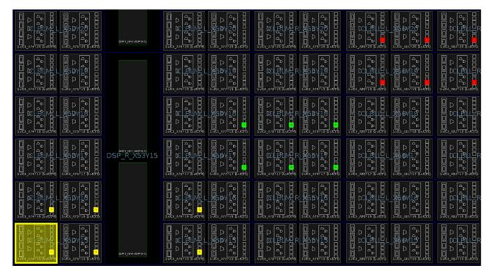
Figure 97: RPM Placement by RLOC\_ORIGIN
