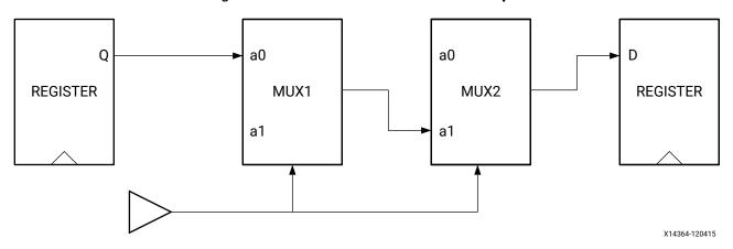
This ensures that all the paths going through the path shown above are selected without needing to find specific patterns for the startpoints and endpoints.
