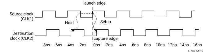
In this example, the setup constraint due to the phase-shift is 0.3 ns. This makes it almost impossible to achieve timing closure. On the other hand, the hold check is -3.7 ns, which is too lenient.
