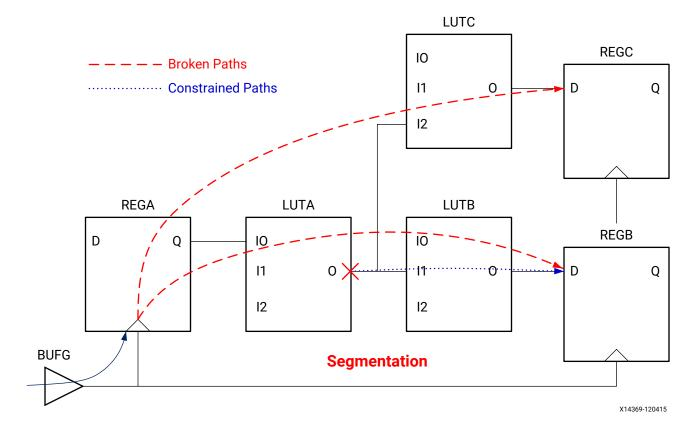
Figure 88: Path Segmentation Breaking Multiple Paths
