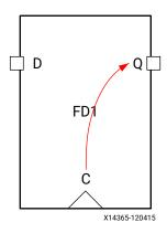
If the constraint is applied to FD1/Q, the timing engine stops the propagation through the arc C->Q to make the pin Q a valid startpoint:
